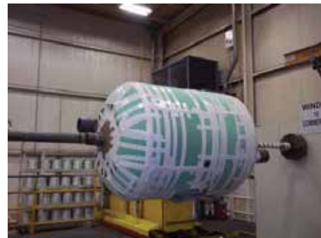
Insulated Vessel at Start of Winding
